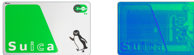
Figure 23: Photograph (left) and processed terahertz image (right) of a Japanese prepaid public transport card, revealing an inside view of the underlying electronics (courtesy of TOPTICA Photonics AG)
