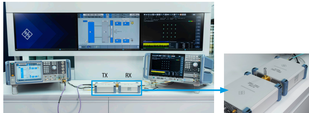
Figure 13: D band (110 GHz to 170 GHz) signal generation and analysis test setup with R&S®FE170ST frontend (transmitter, TX) and R&S®FE170SR frontend (receiver, RX)
